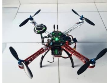
Gambar 5. Hasil rakitan quadcopter
